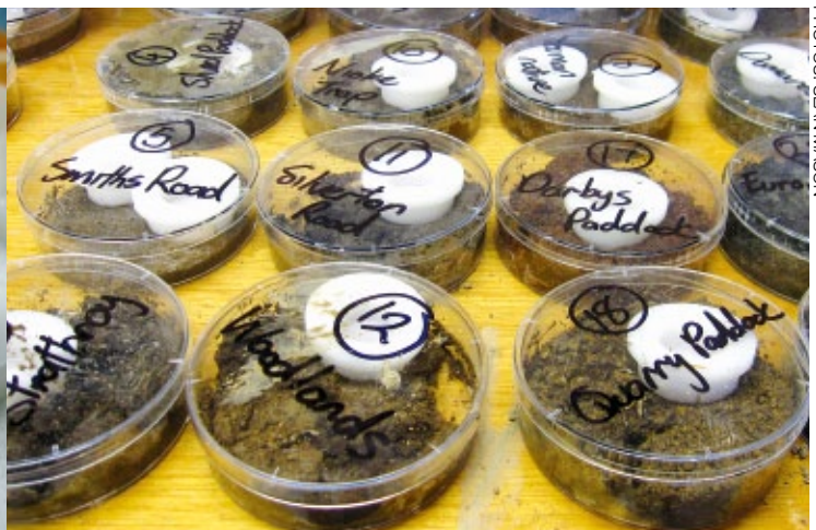
The DGT soil test is a plastic device that attracts available P through a membrane to an iron oxide gel. After 24 hours on moist soil (100 per cent water-holding capacity) the device is washed, and the amount of P bound to the gel is measured.
