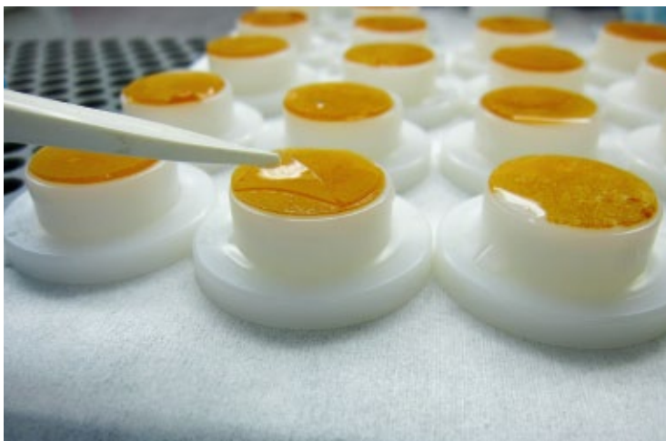
The DGT soil test is a plastic device that attracts available P through a membrane to an iron oxide gel. After 24 hours on moist soil (100 per cent water-holding capacity) the device is washed, and the amount of P bound to the gel is measured.
