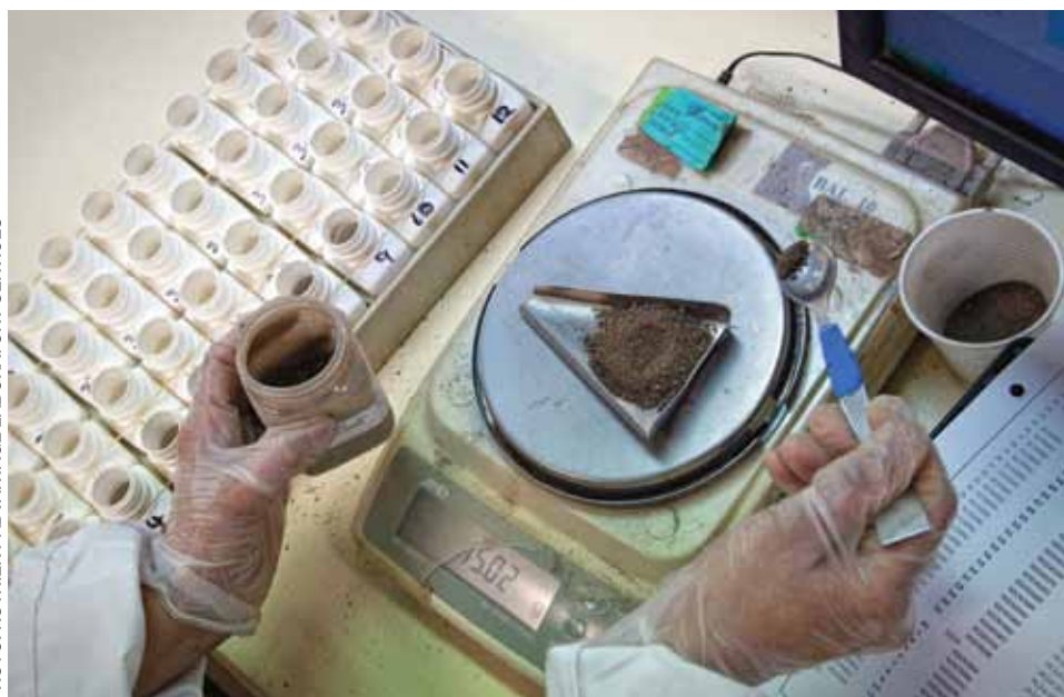
Initial preparation involves weighing soil samples out prior to analysis.
